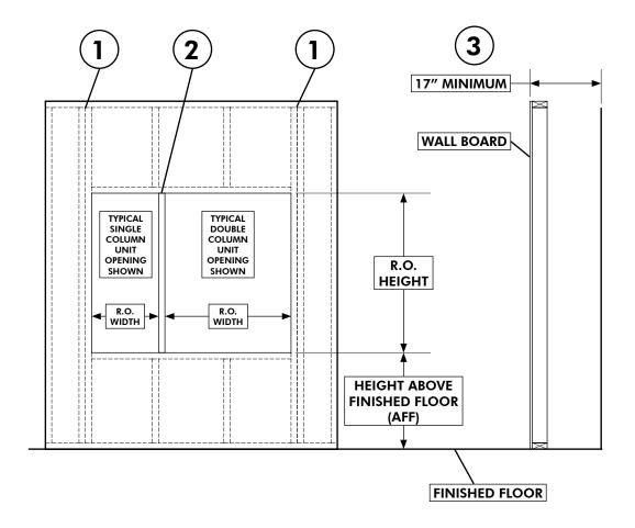
NOTE: All wall frame mounting options are shown for reference only. Refer to local building codes and accessibility regulations to determine proper mounting requirements.
