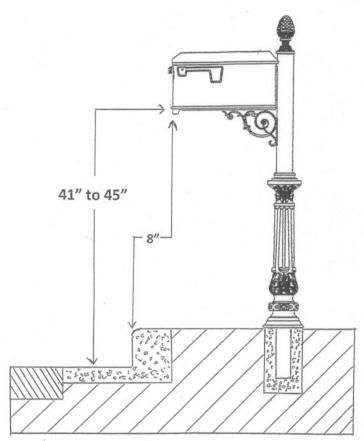
**INSTALLATION:** Assemble entire mailbox unit to post with below instructions. Dig hole approximately 16" deep (this will vary due to local postal codes) with post hole diggers or small shovel. Install completely assembled post into hole and check for fit. Mix quick set style concrete and pack it in around the post in the hole. Level the mailbox post front to back, and side to side off of the round pole. Some temporary supports may be necessary until concrete dries.
