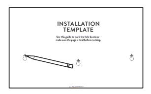
2 Drill into the wall at each marked location. Use a 1/4" drill bit for brick or other masonry wall. Use a 1/16" drill bit for wood wall.
