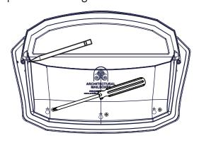
Remove the mailbox from the wall and drill the remaining holes. Insert plastic anchors, if needed.
