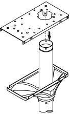
Install the assembled post into the ground. Ensure that the mounting plate is facing toward the street before installing into the ground.
