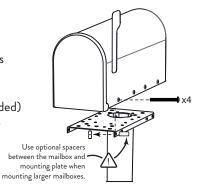
Once the mailbox is mounted, carefully push the plastic bracket up into the mailbox plate. Press the sides of the bracket inward making sure the four studs snap into the rectangular notches on the sides of the mounting plate as shown below.
