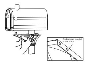
Attach the two halves of the decorative post cover to each other around the post using the 4 small Phillips screws.
