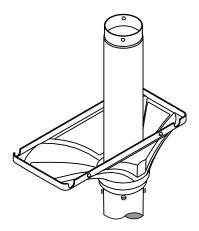
Attach the mounting plate to the post using the 4 small hex bolts, nuts and 8 small washers.
