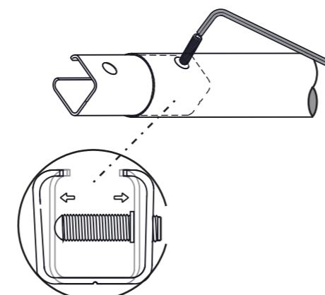
c. Repeat step 1b to properly assemble the second post piece, making sure to minimize the gap between the post pieces.
