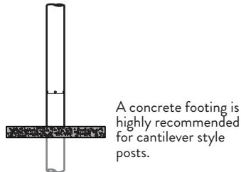
A concrete footing is highly recommended for cantilever style posts.
