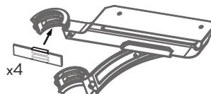
**2b** Locate the correct height for the support arm. According to USPS requirements, the top surface of the arm should rest from 41" to 45" from the road surface.
