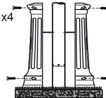
Then, attach the arm to the post using the six medium Phillips screws. Make sure all screws are even and snug.
