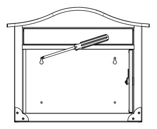
While the mailbox is hanging on the top screws, insert the remaining two screws into the bottom holes and secure with a screwdriver.
